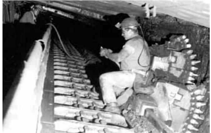
GH 1600 gliding plow at a German Mine in an inclined seam
