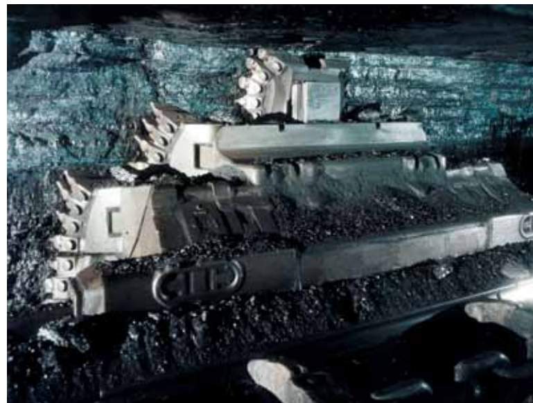
GH1600 gliding plow in hard coal
